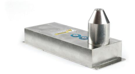
**Model M25:** 50 kV, 4W X-ray Monoblock - The M25 x-ray monoblock is a fully integrated miniature 50 kV, 4W x-ray generator designed specifically to be used as component of a handheld, portable, or bench top x-ray instrument. The source includes a miniature sealed x-ray tube with a transmission-type end window, a high voltage power supply, and control electronics contained in a compact grounded enclosure.
